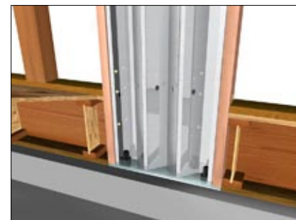
Alternate installation of the first story on a wood-floor system
