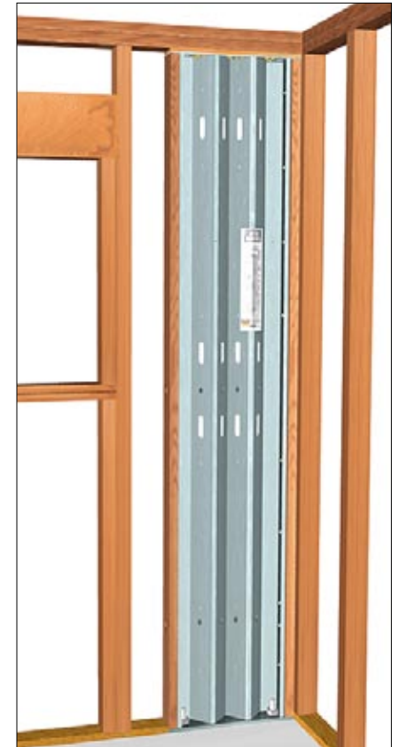
Complete installation of the standard Steel Strong-Wall
