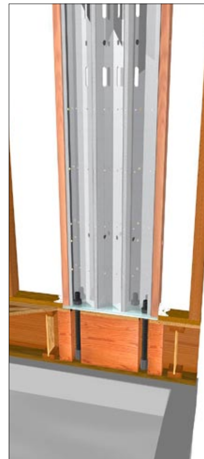
Complete installation of the first story on a wood-floor system
